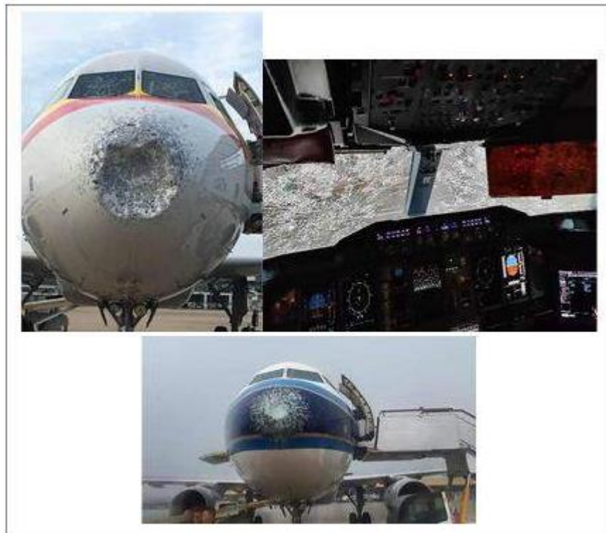
Figure 3. Nose and windshield damage of two aircraft hit by hail stones during the passage of thunderstorms. Left: On July 26th, 2018, Tianjin Airlines flew an Airbus A320 from Tianjin to Haikou. Right and below: On May 26th, 2019, flight No. CZ3101 was flying from Guangzhou to Beijing.
